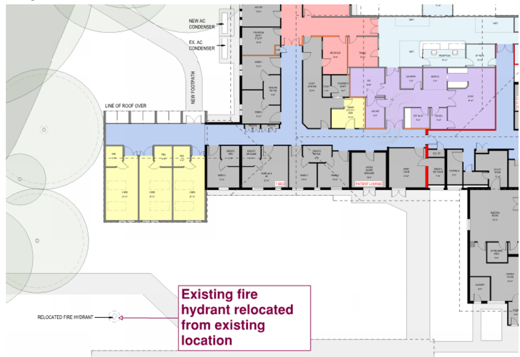
Figure No. 39: Existing external fire hydrant to be relocated because of the proposed redevelopment works.
