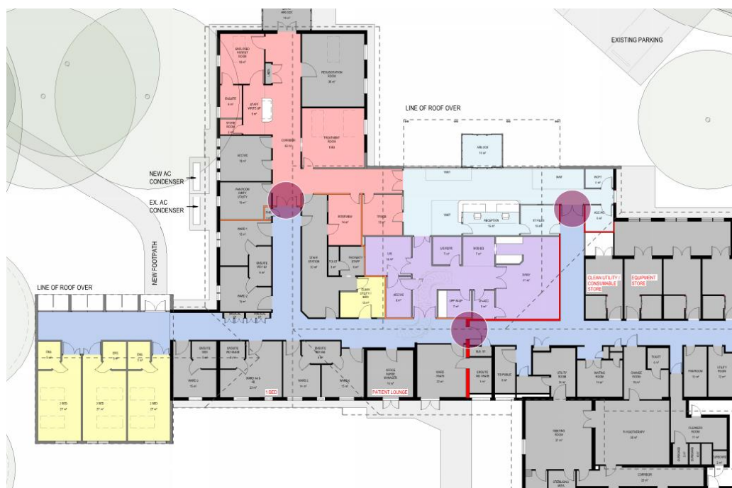
Figure No. 6 – Fire safety doors that swing against the direction of egress
