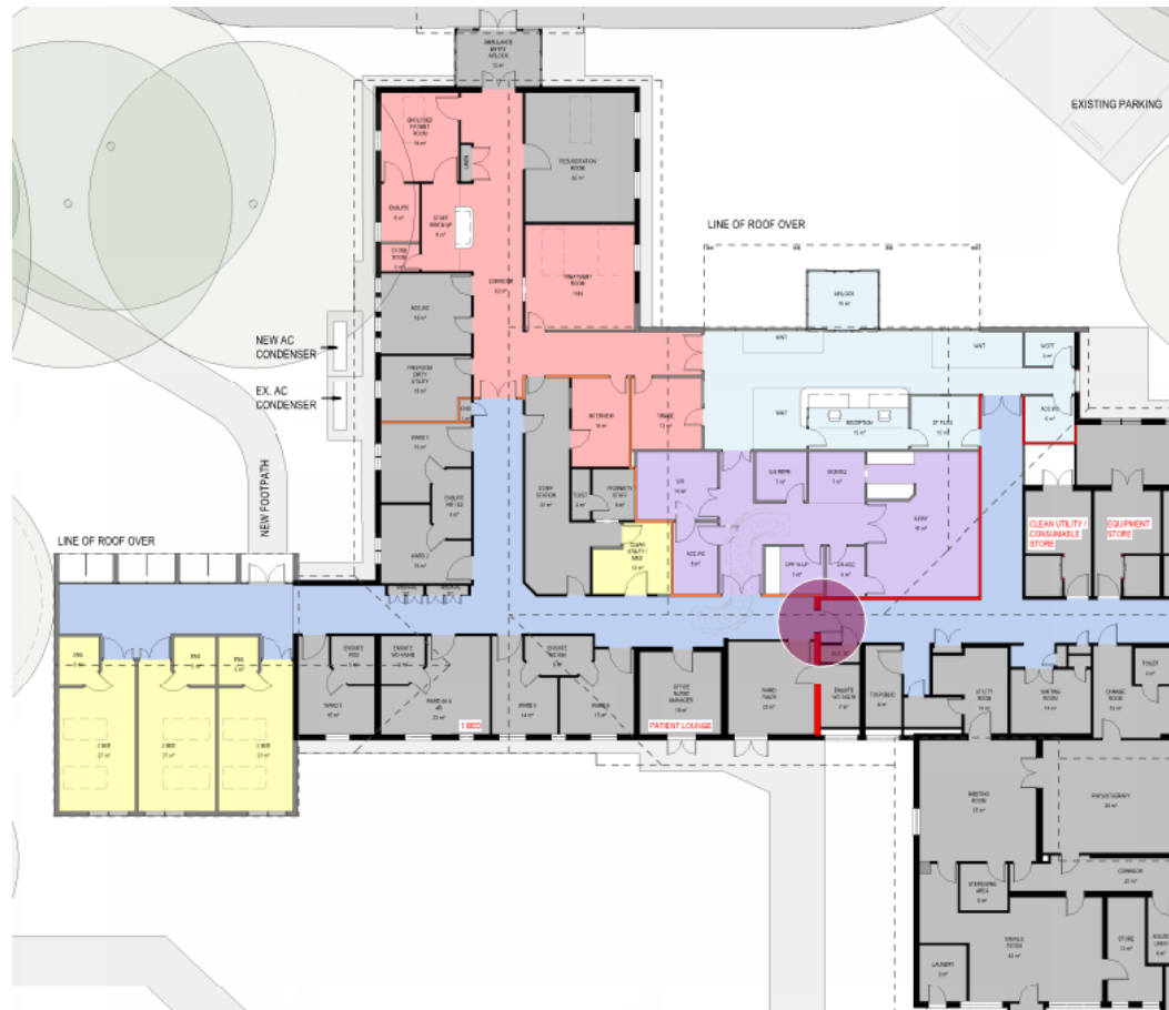
Figure No. 15: Horizontal exit door that does not swing in the direction of egress.
